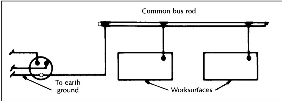
Figure 5. Grounding strategy for workstations without AC power.
