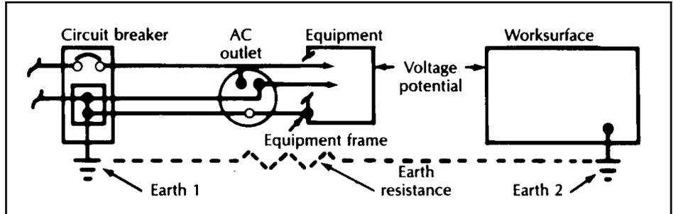
Figure 2. Separate ground systems present potential problems.
