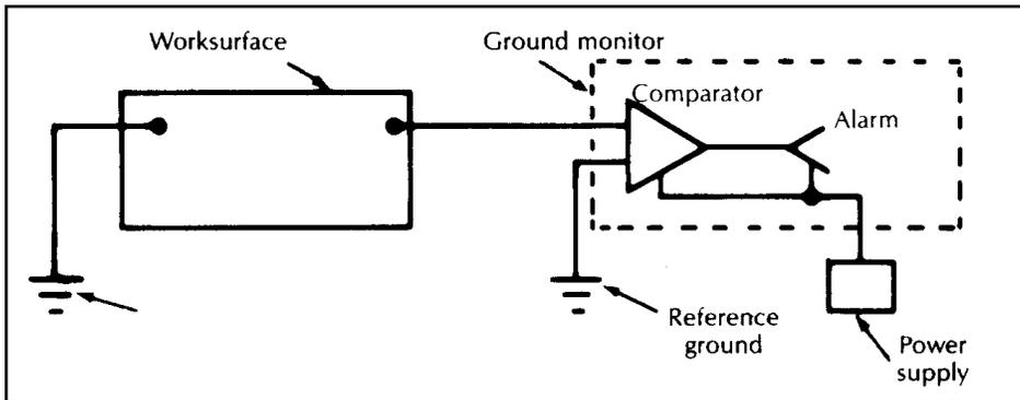
Figure 6. Block diagram of a ground-integrity monitor.
