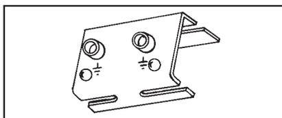
**Figure 2. 13523 premium bench mounted ground with parking station.**
