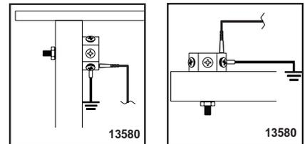
Figure 10. Installation of multi grounding hub.
