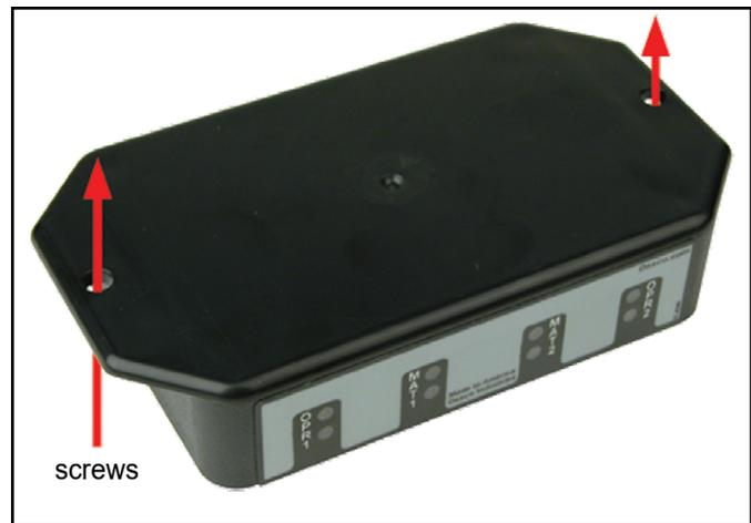
Figure 2. Mounting the Control Unit
