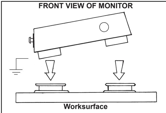
Figure 3. Installation of the monitor to the worksurface one snap at a time.
