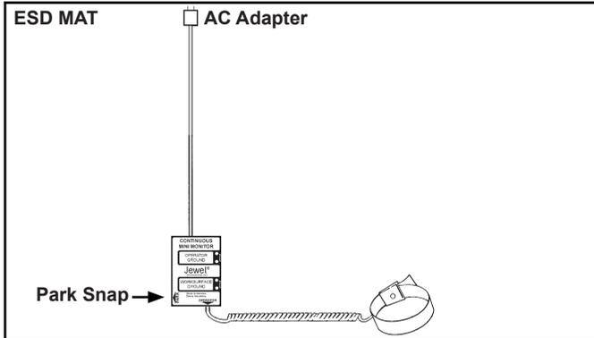
Figure 4. Operating the Jewel® Workstation Continuous Mini Monitor.
