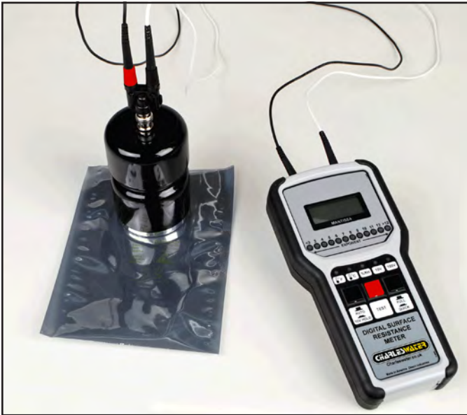
Figure 3. Using the Concentric Ring Probe with the Charleswater Digital Surface Resistance Meter
