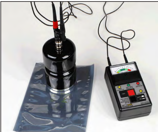
Figure 4. Using the Concentric Ring Probe with the Charleswater Analogue Surface Resistance Meter
