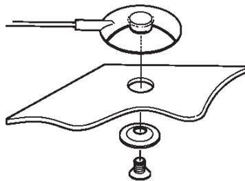
Figure 10. Installing [60286](#) to mat using supplied hardware.
