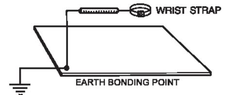
Figure 4. Earth bonding point for each workstation.
