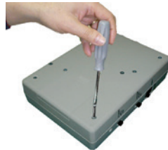
Figure 11: Unscrew The Case
