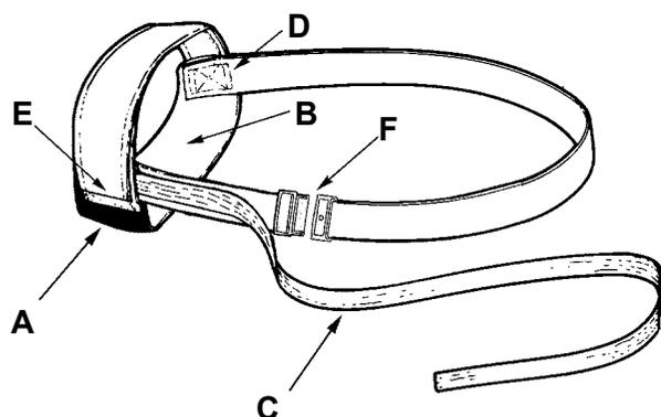
Designed to meet the EN 61340-5-1 footwear requirements tested per IEC 61340-4-3. Per IEC 61340-5-2 paragraph 5.2.8, footwear should be used "where personnel are mobile, in storing areas, operating large machinery, etc., it may be impractical or dangerous to have long cords attached to them."
